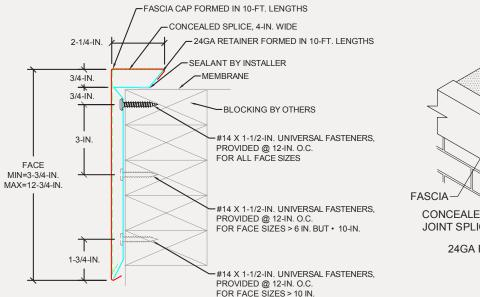
PRE-DRILL WITH 3/16-IN. DRILL BIT FOR MASONRY CONDITIONS. CONTACT US FOR APPROPRIATE RECOMMENDATIONS NEEDED TO MEET/EXCEED ANSI/SPRI/FM4435/ES-1 DESIGN CRITERIA
